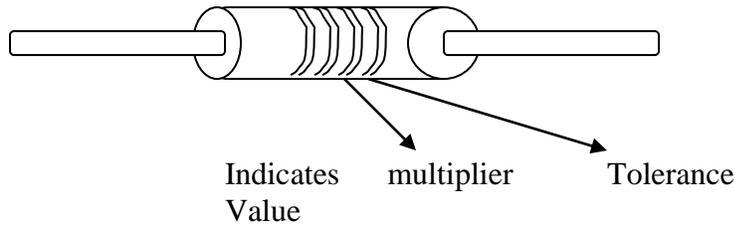
First color band tells the first significant figure of the resistors value.
