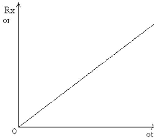
Transmitter Rotor Position Vs Receiver Rotor Position
