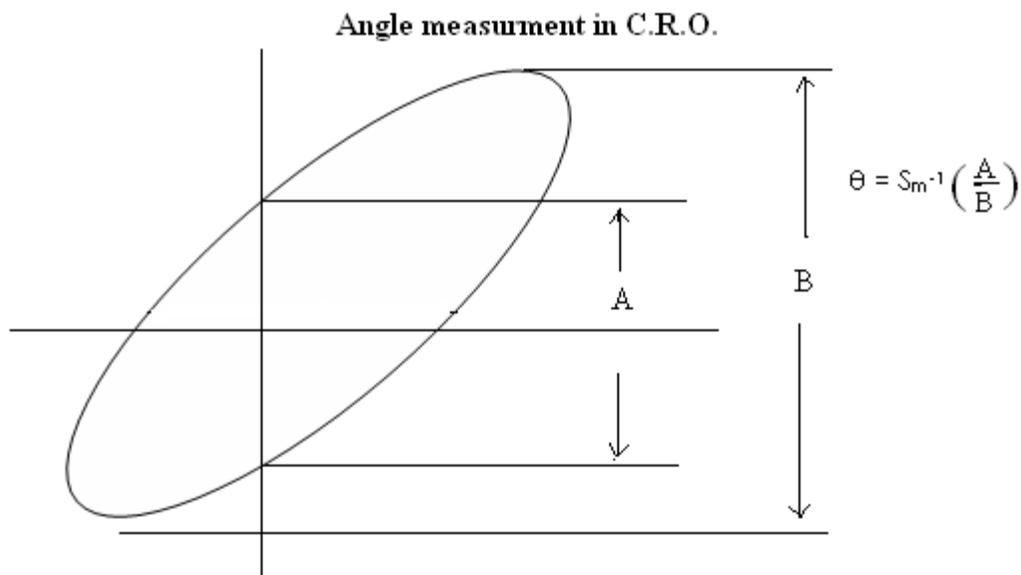
3. C.R.O. is to be connected in X-Y mode for phase displacement measurement connect X-input of CRO to input of lag network and Y- input of C.R.O to output of lag network.
