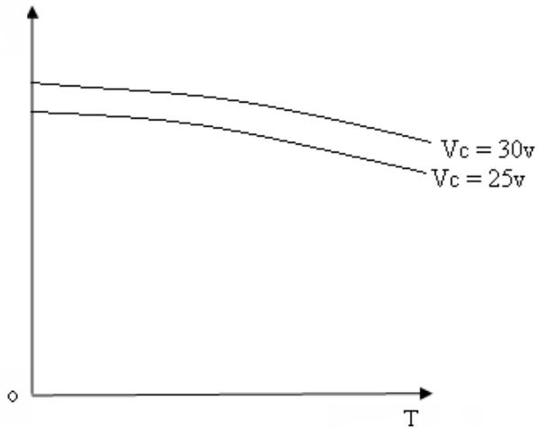
**RESULT:** Speed torque characteristics of AC Servomotor are observed.
